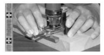
Step 4. Once the slot is cut, assemble the strips and cut them to length with the razor knife or chisel. The corners are cut at a 45 degree angle. Consider making a jig as seen below for this as you will be making many cuts of this type.
